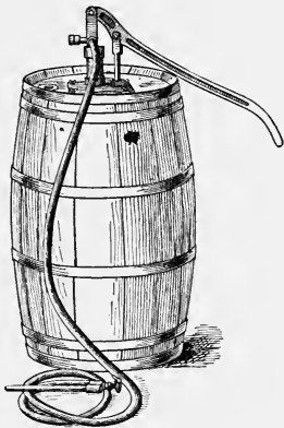
FIG. 45—SUBMERGED BARREL PUMP
